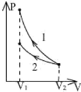
$$A_1 = \frac{RT_1}{\gamma - 1} \frac{m}{M} \left[ 1 - \left( \frac{V_1}{V_2} \right)^{\gamma-1} \right], \quad (1)$$
