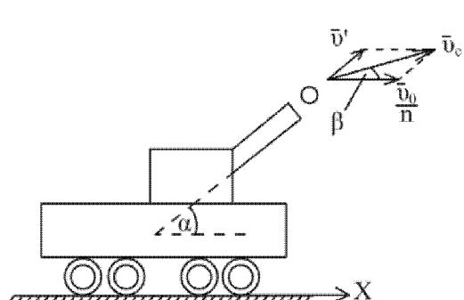
$$(M+m)v_0 = M \frac{v_0}{n} + mv_c \cos \beta,$$
