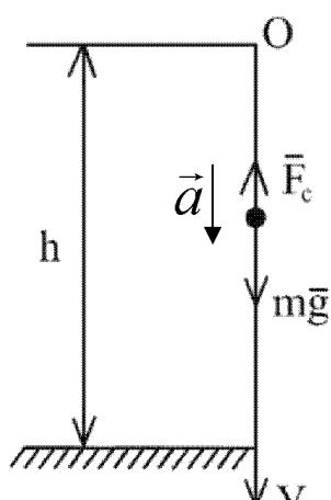
$$ma = mg - F_c \quad \text{или} \quad m \frac{dv}{dt} = mg - rv. \quad (1)$$
