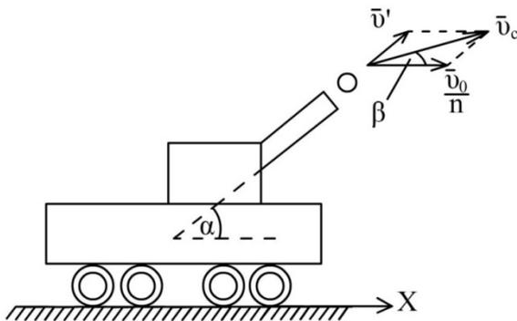
$$(M + m)v_0 = M \frac{v_0}{n} + m v_c \cos \beta,$$
