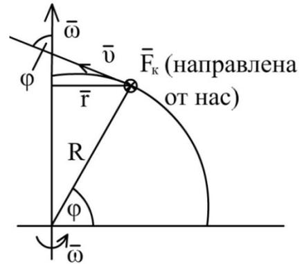
$$F = \frac{4\pi m v \sin \alpha}{T}; \quad [F] = \frac{\text{кг} \cdot \frac{\text{м}}{\text{с}}}{\text{с}} = \frac{\text{кг} \cdot \text{м}}{\text{с}^2} = \text{Н};$$
