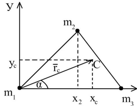
$$x_c = \frac{\sum_{i=1}^n m_i x_i}{\sum_{i=1}^n m_i}; \quad y_c = \frac{\sum_{i=1}^n m_i y_i}{\sum_{i=1}^n m_i},$$
