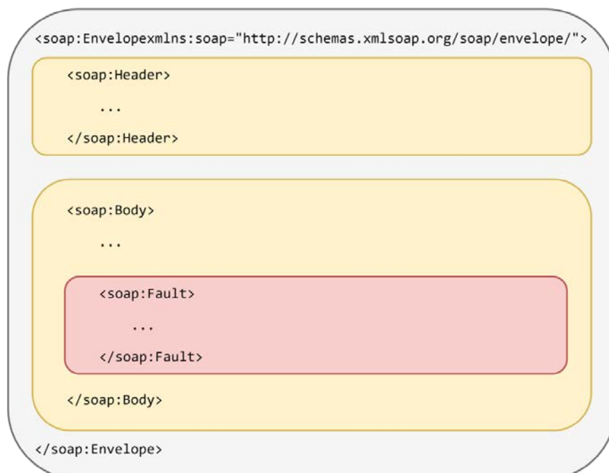
Fig. 1. The Structure of XML Message Transmitted via the SOAP Protocol
