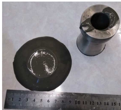
Figure 1. – Determination of cement paste melt with a polymer additive DLP2000
