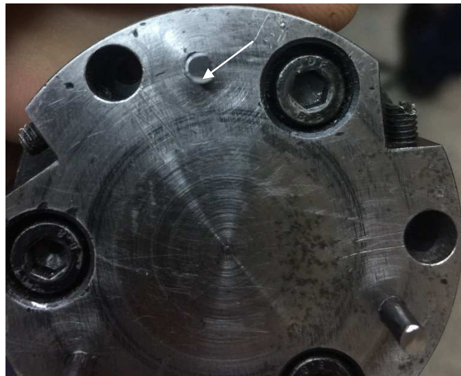
Figure 2. – Dark wear stripes on specimens
