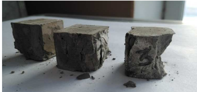
Figure 3. – Samples after testing (with 3% polymer additive Primal CM330)
