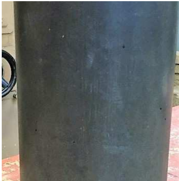
Figure 1. – The homogeneity of the obtained sample of sulfur concrete
