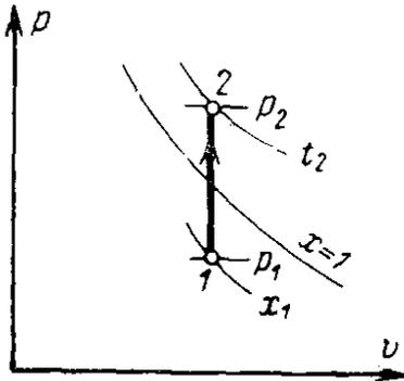
$$q = \Delta u = u_2 - u_1 \quad \text{или} \quad q = i_2 - i_1 - J(p_2 - p_1)$$
