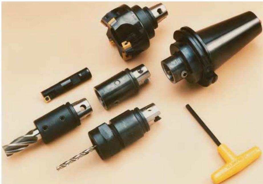
Fig. 4.2. ‘Modular tooling concepts’ allow ‘qualified tooling’ to be set up with the minimum of adjustments, thereby significantly reducing downtime
