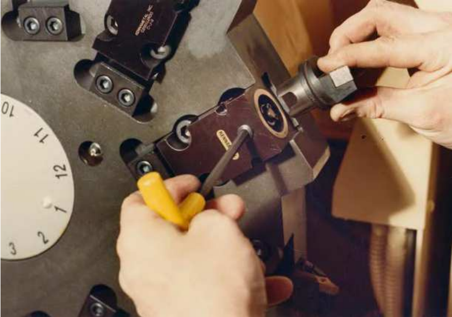
Fig. 4.3. ‘KM’ modular quickchange tooling system being manually- fitted/changed – using the T-bar wrench, into a turning center’s turret
