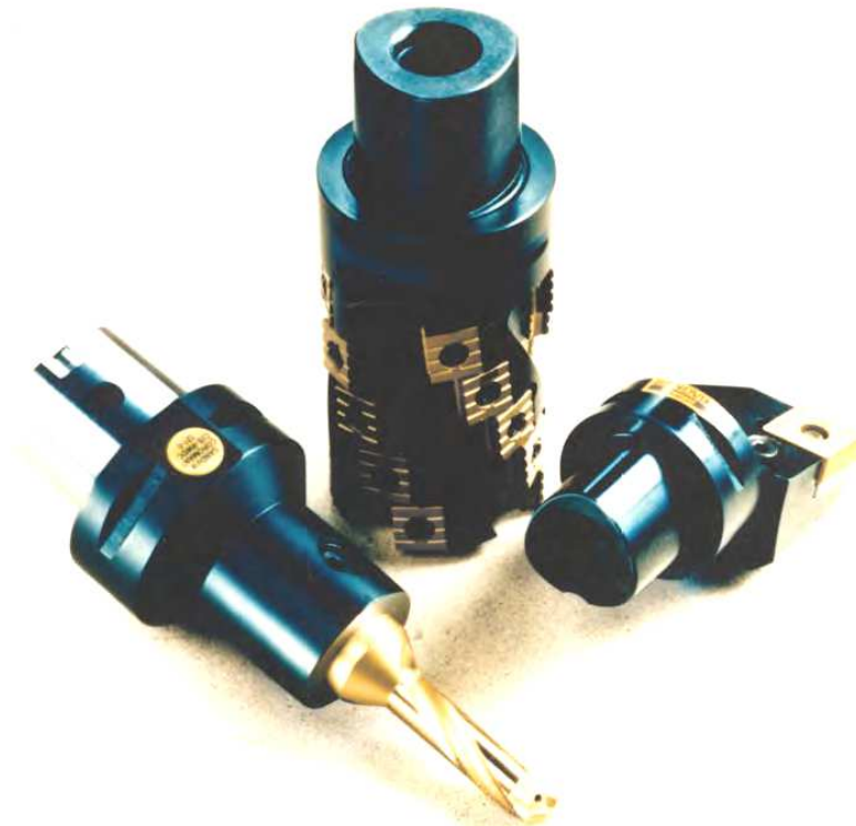
Fig. 4.5. Modular tooling (Capto) illustrating stationary (turning) and rotational tooling (milling, drilling, etc.), with identical lobed and tapered 'back-ends'
