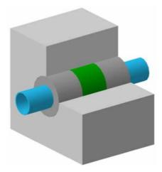
Figure 1. – A joint using a metal sleeve
