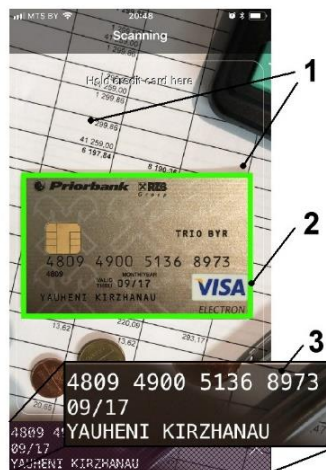
Fig.1. Our mobile app interface for content recognition: 1 - the viewing area; 2 - highlighting of bank card successful detection; 3 - the data output area
