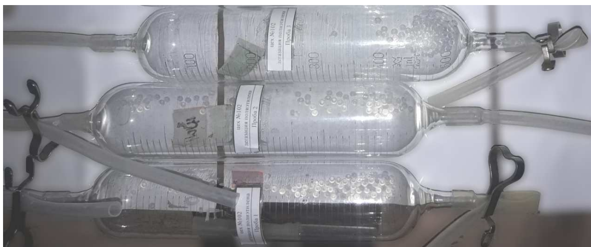
Figure 1. – Degassing of the samples of polyethylene
