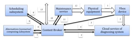
Figure 6. - Scheme of integration of vibration diagnosing system and business management system
