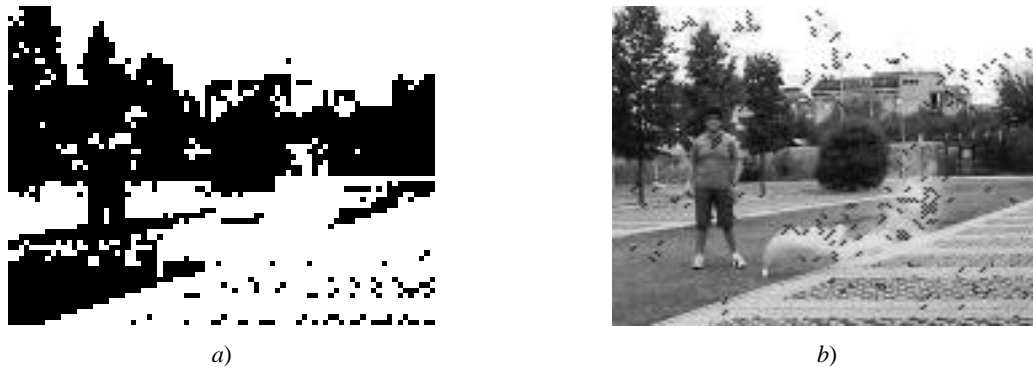
Fig. 3. Otsu threshold mask (a) and the current (b) frame with moving vectors
