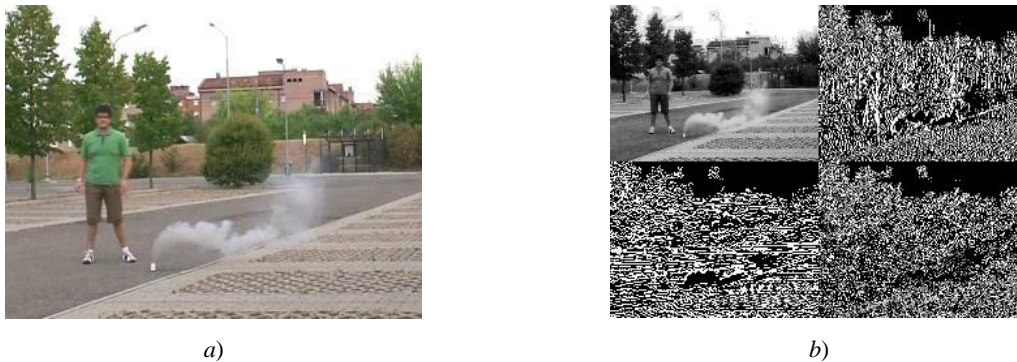
Fig. 1. The current frame (a) and the discrete wavelet transform after grayscale transformation and histogram equalization (b)
