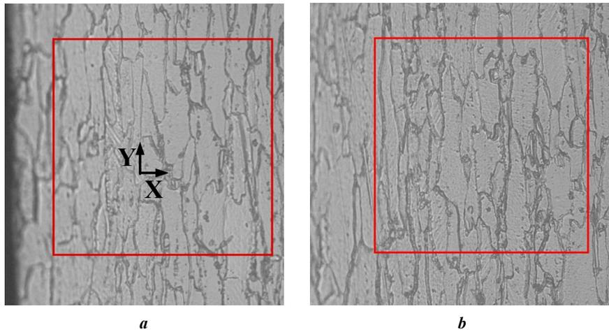
**Fig. 8.** Tinplate microstructure in the thickness sections of the TS 435 steel sheet 0.19 mm thick in the plane along the rolling direction line ( $\times 500$ ):
