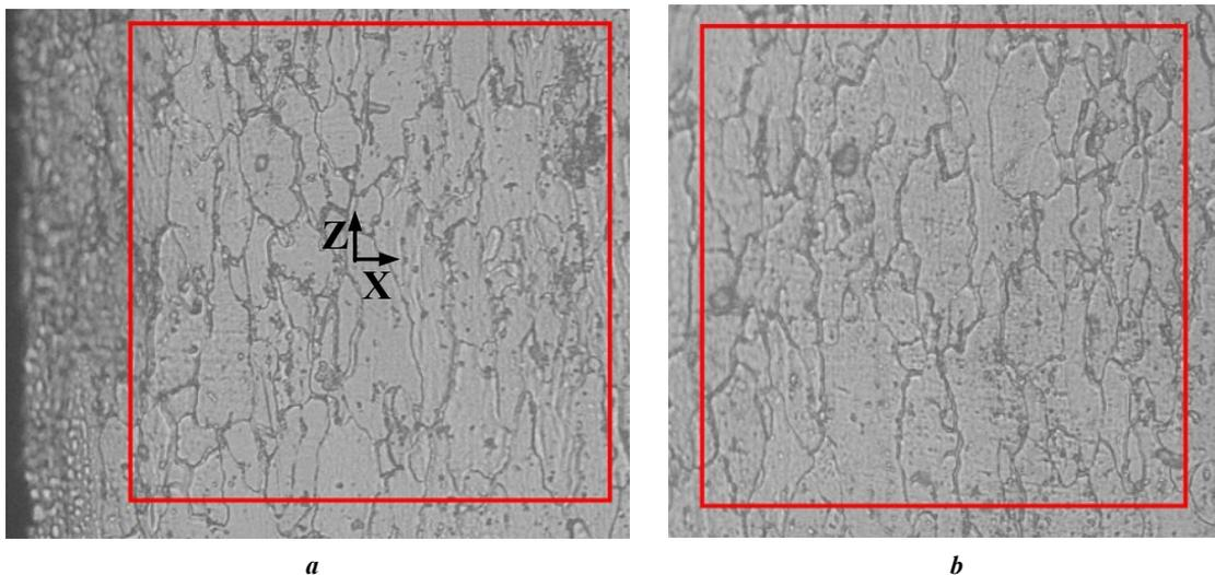
**Fig. 9.** Microstructure of the TS 435 steel tinplate sheet 0.19 mm thick in the plane across the rolling direction line ( $\times 500$ ):
