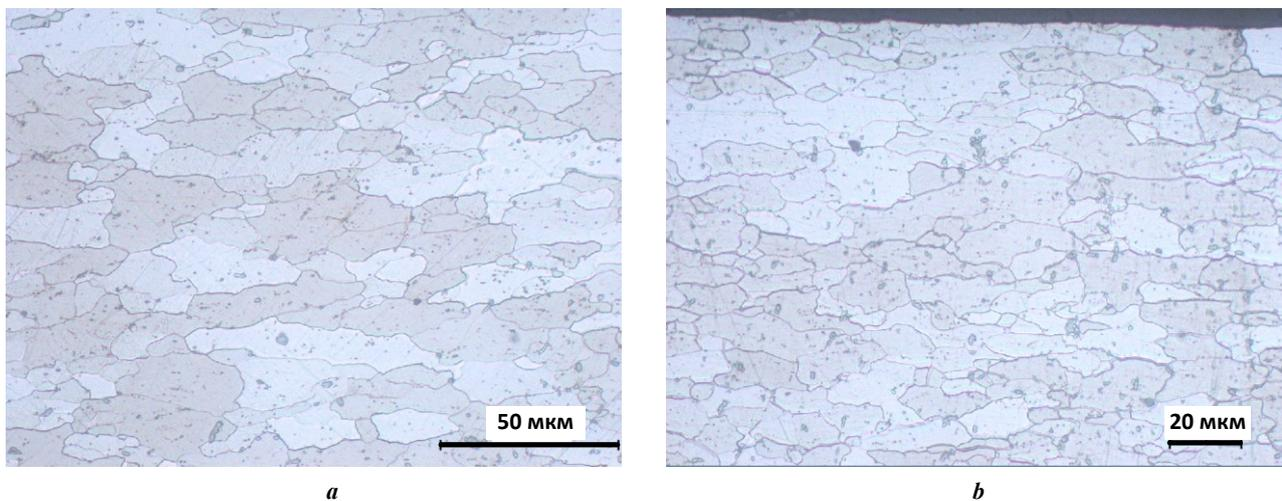
**Fig. 4.** Metal microstructure of an annealed TS 435 steel strip 0.224 mm thick, which is fed to the DSR-1250 mill for skin pass ( $\times 500$ ):
