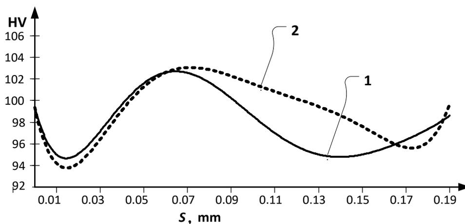
**Fig. 6.** Microhardness distribution along the thickness of the TS 435 steel sheet 0.19 mm thick subjected to skin pass in the DSR-1250 mill, according to the results of measurements on the oblique cut surface: HV – microhardness on the oblique cut surface; S – depth (measurement coordinate) along the sheet thickness; 1 – cross cut measurements; 2 – along cut measurements
