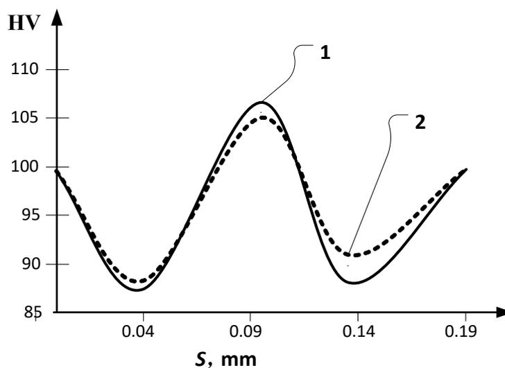
**Fig. 5.** Microhardness distribution along the thickness of the TS 435 steel sheet 0.19 mm thick subjected to skin pass in the DSR-1250 mill, according to the results of measurements from the sheet end face:
