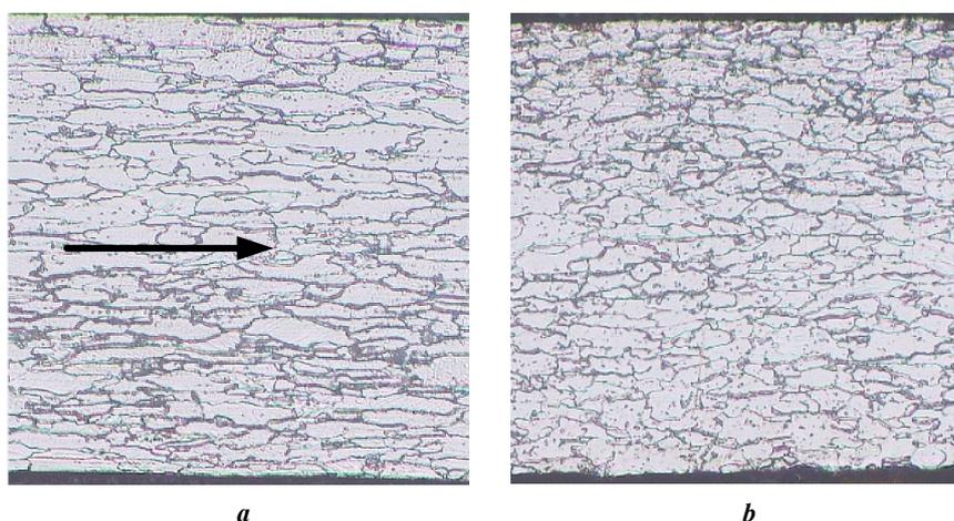
**Fig. 7.** Microstructure of the TS 435 steel tinplate sheet 0.19 mm thick: a – microstructure in the strip thickness section ( $\times 200$ ) along the rolling line (an arrow – the rolling direction); b – microstructure in the strip thickness section ( $\times 200$ ) across the rolling line (the rolling direction – toward us)
