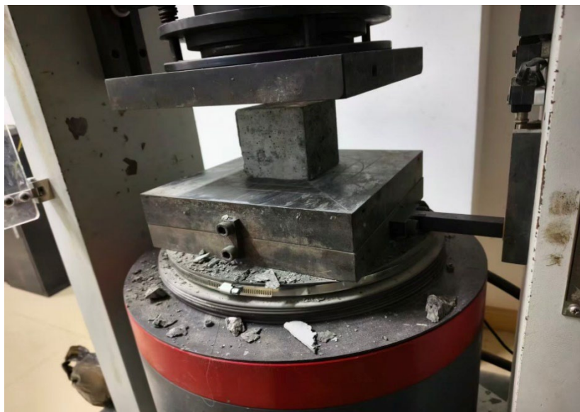
Figure 2. – Example of Servo Hydraulic Compression Testing Machine
